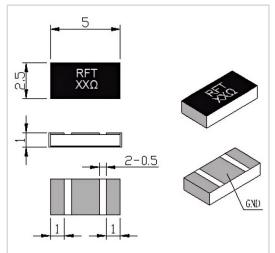
RF Solution offer a wide selection of Chip Resistor for global customers. RFTXXN-20CR2550C is a Chip Resistor in Resistance Range of XX  $\Omega$  (10~3000 $\Omega$ Customizable). It is made of high quality materials under a high standard, the Resistance Tolerance of this product is ±5%, Substrate Material is AIN and Resistive Element is Thick Film. The component has a good working performance and stability, it is ideal for handling a Power of 20 W.
