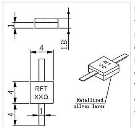
RF Solution offer a wide selection of Leaded Resistor for global customers. RFTXXN-10RM0404 is a Leaded Resistor in Capacitance of 2.3 PF@100 $\Omega$ . It is made of high quality materials under a high standard, the Resistance Range of this product is XX  $\Omega$  (10-3000 $\Omega$ Customizable), Resistance Tolerance is ±5% and Temperature Coefficient Max is 150 ppm/°C. The component has a good working performance and stability, it is ideal for handling a Power of 10 W.
