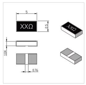
RF Solution offer a wide selection of Chip Resistor for global customers. RFTXXN-10CR2550TA is a Chip Resistor in Resistance Range of XX  $\Omega$  ( $10\sim3000\Omega$  Customizable). It is made of high quality materials under a high standard, the Resistance Tolerance of this product is  $\pm5\%$ , Substrate Material is Al2O3 and Resistive Element is Thick Film. The component has a good working performance and stability, it is ideal for handling a Power of 10 W.
