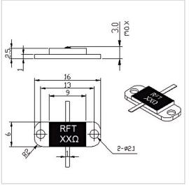
RF Solution offer a wide selection of Flanged Resistor for global customers. RFTXXN-100RJ1606B is a Flanged Resistor in Capacitance of 2.1 PF@100 $\Omega$ . It is made of high quality materials under a high standard, the Resistance of this product is XX  $\Omega$  (10~1500 $\Omega$  Customizable), Resistance Tolerance is  $\pm 5\%$  and Temperature Coefficient Max is 150 ppm/°C. The component has a good working performance and stability, it is ideal for handling a Power of 100 W.
