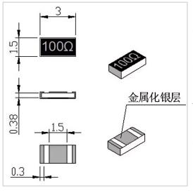
RF Solution offer a wide selection of Chip Resistor for global customers. RFTXXN-05CR1530C is a Chip Resistor in Resistance Range of XX  $\Omega$  (10~3000 $\Omega$  Customizable). It is made of high quality materials under a high standard, the Resistance Tolerance of this product is  $\pm 5\%$ , Substrate Material is AlN and Resistive Element is Thick Film. The component has a good working performance and stability, it is ideal for handling a Power of 5 W.
