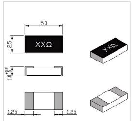
RF Solution offer a wide selection of Chip Resistor for global customers. RFTXXN-02CR2550B is a Chip Resistor in Resistance Range of XX  $\Omega$  (10~3000 $\Omega$ Customizable). It is made of high quality materials under a high standard, the Resistance Tolerance of this product is ±5%, Substrate Material is AIN and Resistive Element is Thick Film. The component has a good working performance and stability, it is ideal for handling a Power of 2 W.
