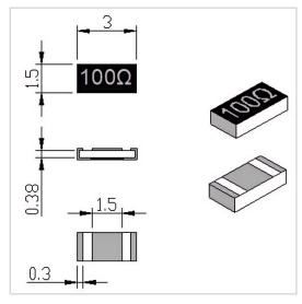
RF Solution offer a wide selection of Chip Resistor for global customers. RFTXXN-02CR1530C is a Chip Resistor in Resistance Range of XX  $\Omega$  (10~3000 $\Omega$  Customizable). It is made of high quality materials under a high standard, the Resistance Tolerance of this product is  $\pm 5\%$ , Substrate Material is AlN and Resistive Element is Thick Film. The component has a good working performance and stability, it is ideal for handling a Power of 2 W.
