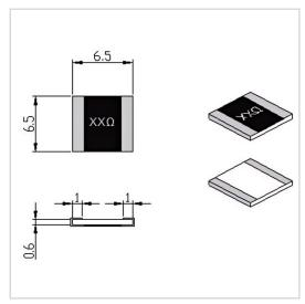
RF Solution offer a wide selection of Chip Resistor for global customers. RFTXXA-05CR6565B is a Chip Resistor in Resistance Range of XX  $\Omega$  ( $10\sim3000\Omega$  Customizable). It is made of high quality materials under a high standard, the Resistance Tolerance of this product is  $\pm5\%$ , Substrate Material is Al2O3 and Resistive Element is Thick Film. The component has a good working performance and stability, it is ideal for handling a Power of 5 W.
