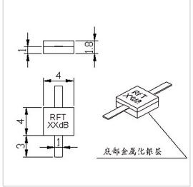
RF Solution offer a wide selection of Leaded Attenuator for global customers. RFTXXA-05AM0404-3 is a Leaded Attenuator in Frequency Range of DC $\sim$ 3.0 GHz. It is made of high quality materials under a high standard, the Attenuation Value of this product is  $01-10 \, dB@15,17,20 \, dB@25,30 \, dB$ , Attenuation Tolerance is  $0\pm0.6 \, dB@\pm0.8 \, dB@\pm1.0dB$  and VSWR Max is 1.20. The component has a good working performance and stability, it is ideal for handling a Rated Power of 5 W.
