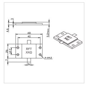
RF Solution offer a wide selection of Flanged Resistor for global customers. RFTXX-800RM4826 is a Flanged Resistor in Capacitance of 21.8 PF@100 $\Omega$ . It is made of high quality materials under a high standard, the Resistance of this product is XX  $\Omega$  (Customizable), Resistance Tolerance is  $\pm 5\%$  and Temperature Coefficient Max is 150 ppm/°C. The component has a good working performance and stability, it is ideal for handling a Power of 800 W.
