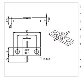
RF Solution offer a wide selection of Flanged Resistor for global customers. RFTXX-60RM2006 is a Flanged Resistor in Capacitance of 2.6 PF@100 $\Omega$ . It is made of high quality materials under a high standard, the Resistance of this product is XX  $\Omega$  (10~2000 $\Omega$ Customizable), Resistance Tolerance is ±5% and Temperature Coefficient Max is 150 ppm/°C. The component has a good working performance and stability, it is ideal for handling a Power of 60 W.
