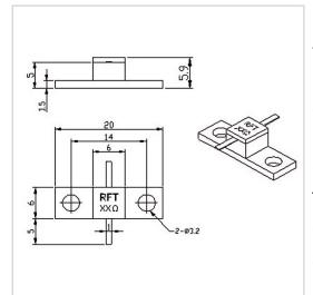
RF Solution offer a wide selection of Flanged Resistor for global customers. RFTXX-60RM2006F is a Flanged Resistor in Capacitance of 1.2 PF@100 $\Omega$ . It is made of high quality materials under a high standard, the Resistance of this product is XX  $\Omega$  (10~2000 $\Omega$ Customizable), Resistance Tolerance is ±5% and Temperature Coefficient Max is 150 ppm/°C. The component has a good working performance and stability, it is ideal for handling a Power of 60 W.
