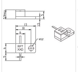
RF Solution offer a wide selection of Flanged Resistor for global customers. RFTXX-60RM1306F is a Flanged Resistor in Capacitance of 1.2 PF@100 $\Omega$ . It is made of high quality materials under a high standard, the Resistance of this product is XX  $\Omega$  (10~2000 $\Omega$ Customizable), Resistance Tolerance is ±5% and Temperature Coefficient Max is 150 ppm/°C. The component has a good working performance and stability, it is ideal for handling a Power of 60 W.
