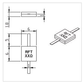
RF Solution offer a wide selection of Leaded Resistor for global customers. RFTXX-60RM0606 is a Leaded Resistor in Capacitance of 2.6 PF@100 $\Omega$ . It is made of high quality materials under a high standard, the Resistance Range of this product is XX  $\Omega$  (10-3000 $\Omega$  Customizable), Resistance Tolerance is  $\pm 5\%$  and Temperature Coefficient Max is 150 ppm/°C. The component has a good working performance and stability, it is ideal for handling a Power of 60 W.
