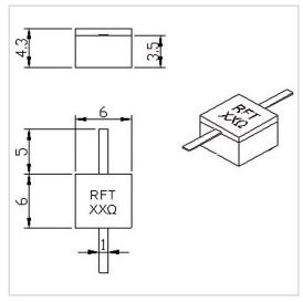
RF Solution offer a wide selection of Leaded Resistor for global customers. RFTXX-60RM0606F is a Leaded Resistor in Capacitance of 1.2 PF@100 $\Omega$ . It is made of high quality materials under a high standard, the Resistance Range of this product is XX  $\Omega$  (10-3000 $\Omega$  Customizable), Resistance Tolerance is  $\pm 5\%$  and Temperature Coefficient Max is 150 ppm/°C. The component has a good working performance and stability, it is ideal for handling a Power of 60 W.
