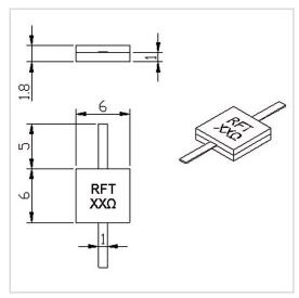
RF Solution offer a wide selection of Leaded Resistor for global customers. RFTXX-60RM0606-2 is a Leaded Resistor in Capacitance of 2.9 PF@100 $\Omega$ . It is made of high quality materials under a high standard, the Resistance Range of this product is XX  $\Omega$  (10-3000 $\Omega$  Customizable), Resistance Tolerance is  $\pm 5\%$  and Temperature Coefficient Max is 150 ppm/°C. The component has a good working performance and stability, it is ideal for handling a Power of 60 W.
