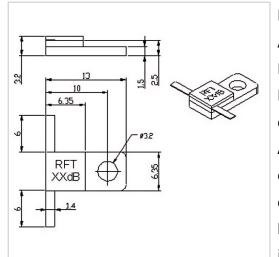
RF Solution offer a wide selection of Flanged Attenuator for global customers. RFTXX-60AM1663B-3 is a Flanged Attenuator in Frequency Range of DC~3.0 GHz. It is made of high quality materials under a high standard, the Attenuation Value of this product is 01-10 dBdB320 dB, Attenuation Tolerance is  $0\pm0.6 \text{ dB}$ dB $3\pm1.0 \text{ dB}$  and VSWR Max is 1.25. The component has a good working performance and stability, it is ideal for handling a Rated Power of 60 W.
