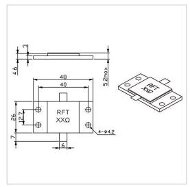
RF Solution offer a wide selection of Flanged Resistor for global customers. RFTXX-600RM4826 is a Flanged Resistor in Capacitance of 21.8 PF@100 $\Omega$ . It is made of high quality materials under a high standard, the Resistance of this product is XX  $\Omega$  (Customizable), Resistance Tolerance is  $\pm 5\%$  and Temperature Coefficient Max is 150 ppm/°C. The component has a good working performance and stability, it is ideal for handling a Power of 600 W.
