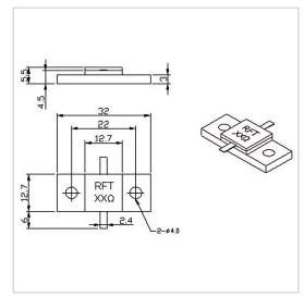
RF Solution offer a wide selection of Flanged Resistor for global customers. RFTXX-500RM3213 is a Flanged Resistor in Capacitance of 8.5 PF@100 $\Omega$ . It is made of high quality materials under a high standard, the Resistance of this product is XX  $\Omega$  (10~1000 $\Omega$  Customizable), Resistance Tolerance is  $\pm 5\%$  and Temperature Coefficient Max is 150 ppm/°C. The component has a good working performance and stability, it is ideal for handling a Power of 500 W.
