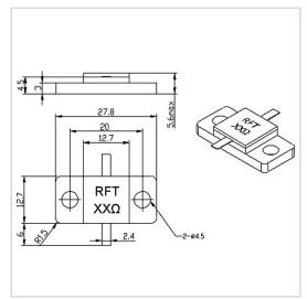
RF Solution offer a wide selection of Flanged Resistor for global customers. RFTXX-500RM2813 is a Flanged Resistor in Capacitance of 8.5 PF@100 $\Omega$ . It is made of high quality materials under a high standard, the Resistance of this product is XX  $\Omega$  (10~1000 $\Omega$  Customizable), Resistance Tolerance is  $\pm 5\%$  and Temperature Coefficient Max is 150 ppm/°C. The component has a good working performance and stability, it is ideal for handling a Power of 500 W.
