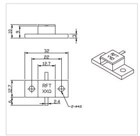
RF Solution offer a wide selection of Flanged Resistor for global customers. RFTXX-400RM3213K is a Flanged Resistor in Capacitance of 2.0 PF@100 $\Omega$ . It is made of high quality materials under a high standard, the Resistance of this product is XX  $\Omega$  (10~1000 $\Omega$  Customizable), Resistance Tolerance is  $\pm 5\%$  and Temperature Coefficient Max is 150 ppm/°C. The component has a good working performance and stability, it is ideal for handling a Power of 400 W.
