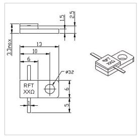
RF Solution offer a wide selection of Flanged Resistor for global customers. RFTXX-30RM1306 is a Flanged Resistor in Capacitance of 2.6 PF@100 $\Omega$ . It is made of high quality materials under a high standard, the Resistance of this product is XX  $\Omega$  (10~2000 $\Omega$  Customizable), Resistance Tolerance is  $\pm 5\%$  and Temperature Coefficient Max is 150 ppm/°C. The component has a good working performance and stability, it is ideal for handling a Power of 30 W.
