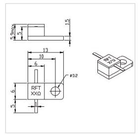
RF Solution offer a wide selection of Flanged Resistor for global customers. RFTXX-30RM1306F is a Flanged Resistor in Capacitance of 1.2 PF@100 $\Omega$ . It is made of high quality materials under a high standard, the Resistance of this product is XX  $\Omega$  (10~2000 $\Omega$  Customizable), Resistance Tolerance is  $\pm 5\%$  and Temperature Coefficient Max is 150 ppm/°C. The component has a good working performance and stability, it is ideal for handling a Power of 30 W.
