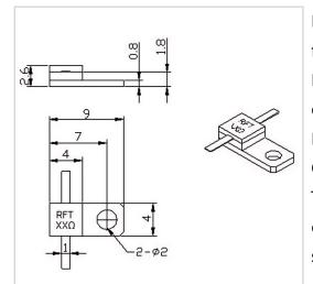
RF Solution offer a wide selection of Flanged Resistor for global customers. RFTXX-30RM0904 is a Flanged Resistor in Capacitance of 1.2 PF@100 $\Omega$ . It is made of high quality materials under a high standard, the Resistance of this product is XX  $\Omega$  (10~2000 $\Omega$ Customizable), Resistance Tolerance is ±5% and Temperature Coefficient Max is 150 ppm/°C. The component has a good working performance and stability, it is ideal for handling a Power of 30 W.
