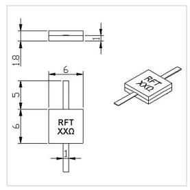
RF Solution offer a wide selection of Leaded Resistor for global customers. RFTXX-30RM0606 is a Leaded Resistor in Capacitance of 2.6 PF@100 $\Omega$ . It is made of high quality materials under a high standard, the Resistance Range of this product is XX  $\Omega$  (10-3000 $\Omega$  Customizable), Resistance Tolerance is  $\pm 5\%$  and Temperature Coefficient Max is 150 ppm/°C. The component has a good working performance and stability, it is ideal for handling a Power of 30 W.
