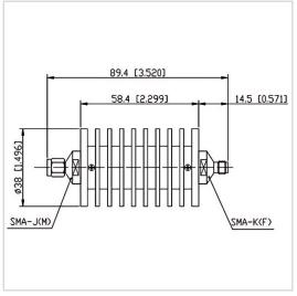
RF Solution offer a wide selection of Coaxial Fixed Attenuator for global customers. RFTXX-30RA3858-SMA-18 is Coaxial Fixed Attenuator in Frequency Range of DC~18.0GHz. It is made of high quality materials under a high standard, the VSWR Max of this product is 1.40, Attenuation Value is 3, 6, 10, 20, 30, 40 dB and Attenuation Tolerance is -1.5dB/+2.0 dB. The component has a good working performance and stability, it is ideal for handling a Power of 30 W.
