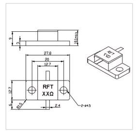
RF Solution offer a wide selection of Flanged Resistor for global customers. RFTXX-300RM2813K is a Flanged Resistor in Capacitance of 2.0 PF@100 $\Omega$ . It is made of high quality materials under a high standard, the Resistance of this product is XX  $\Omega$  (10~1000 $\Omega$  Customizable), Resistance Tolerance is  $\pm 5\%$  and Temperature Coefficient Max is 150 ppm/°C. The component has a good working performance and stability, it is ideal for handling a Power of 300 W.
