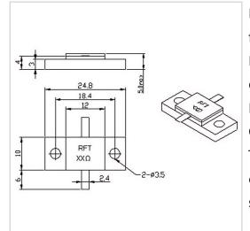
RF Solution offer a wide selection of Flanged Resistor for global customers. RFTXX-300RM2510 is a Flanged Resistor in Capacitance of 5.0 PF@100 $\Omega$ . It is made of high quality materials under a high standard, the Resistance of this product is XX  $\Omega$  (10~1000 $\Omega$ Customizable), Resistance Tolerance is ±5% and Temperature Coefficient Max is 150 ppm/°C. The component has a good working performance and stability, it is ideal for handling a Power of 300 W.
