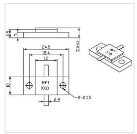
RF Solution offer a wide selection of Flanged Resistor for global customers. RFTXX-300RM2510B is a Flanged Resistor in Capacitance of 4.0 PF@100 $\Omega$ . It is made of high quality materials under a high standard, the Resistance of this product is XX  $\Omega$  (10~1000 $\Omega$  Customizable), Resistance Tolerance is  $\pm 5\%$  and Temperature Coefficient Max is 150 ppm/°C. The component has a good working performance and stability, it is ideal for handling a Power of 300 W.
