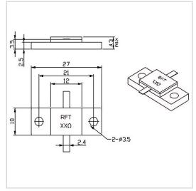
RF Solution offer a wide selection of Flanged Resistor for global customers. RFTXX-250RM2710 is a Flanged Resistor in Capacitance of 5.0 PF@100 $\Omega$ . It is made of high quality materials under a high standard, the Resistance of this product is XX  $\Omega$  (10~1000 $\Omega$  Customizable), Resistance Tolerance is  $\pm 5\%$  and Temperature Coefficient Max is 150 ppm/°C. The component has a good working performance and stability, it is ideal for handling a Power of 250 W.
