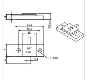
RF Solution offer a wide selection of Flanged Resistor for global customers. RFTXX-250RM2510 is a Flanged Resistor in Capacitance of 5.0 PF@100 $\Omega$ . It is made of high quality materials under a high standard, the Resistance of this product is XX  $\Omega$  (10~1000 $\Omega$ Customizable), Resistance Tolerance is ±5% and Temperature Coefficient Max is 150 ppm/°C. The component has a good working performance and stability, it is ideal for handling a Power of 250 W.
