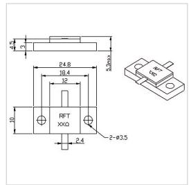
RF Solution offer a wide selection of Flanged Resistor for global customers. RFTXX-250RM2510B is a Flanged Resistor in Capacitance of 4.0 PF@100 $\Omega$ . It is made of high quality materials under a high standard, the Resistance of this product is XX  $\Omega$  (10~1000 $\Omega$  Customizable), Resistance Tolerance is  $\pm 5\%$  and Temperature Coefficient Max is 150 ppm/°C. The component has a good working performance and stability, it is ideal for handling a Power of 250 W.
