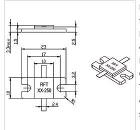
RF Solution offer a wide selection of Flanged Resistor for global customers. RFTXX-250RM2310 is a Flanged Resistor in Capacitance of 5.6 PF@100 $\Omega$ . It is made of high quality materials under a high standard, the Resistance of this product is XX  $\Omega$  (10~1500 $\Omega$ Customizable), Resistance Tolerance is ±5% and Temperature Coefficient Max is 150 ppm/°C. The component has a good working performance and stability, it is ideal for handling a Power of 250 W.
