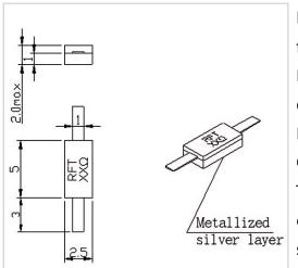
RF Solution offer a wide selection of Leaded Resistor for global customers. RFTXX-20RM2550 is a Leaded Resistor in Capacitance of 1.8 PF@100 $\Omega$ . It is made of high quality materials under a high standard, the Resistance Range of this product is XX  $\Omega$  (10-3000 $\Omega$ Customizable), Resistance Tolerance is ±5% and Temperature Coefficient Max is 150 ppm/°C. The component has a good working performance and stability, it is ideal for handling a Power of 20 W.
