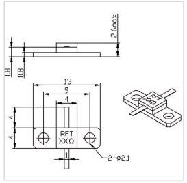
RF Solution offer a wide selection of Flanged Resistor for global customers. RFTXX-20RM1304 is a Flanged Resistor in Capacitance of 1.2 PF@100 $\Omega$ . It is made of high quality materials under a high standard, the Resistance of this product is XX  $\Omega$  (10~3000 $\Omega$  Customizable), Resistance Tolerance is  $\pm 5\%$  and Temperature Coefficient Max is 150 ppm/°C. The component has a good working performance and stability, it is ideal for handling a Power of 20 W.
