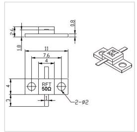
RF Solution offer a wide selection of Flanged Resistor for global customers. RFTXX-20RM1104 is a Flanged Resistor in Capacitance of 1.2 PF@100 $\Omega$ . It is made of high quality materials under a high standard, the Resistance of this product is XX  $\Omega$  (10~3000 $\Omega$  Customizable), Resistance Tolerance is  $\pm 5\%$  and Temperature Coefficient Max is 150 ppm/°C. The component has a good working performance and stability, it is ideal for handling a Power of 20 W.
