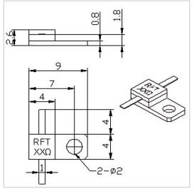
RF Solution offer a wide selection of Flanged Resistor for global customers. RFTXX-20RM0904 is a Flanged Resistor in Capacitance of 1.2 PF@100 $\Omega$ . It is made of high quality materials under a high standard, the Resistance of this product is XX  $\Omega$  (10~3000 $\Omega$  Customizable), Resistance Tolerance is  $\pm 5\%$  and Temperature Coefficient Max is 150 ppm/°C. The component has a good working performance and stability, it is ideal for handling a Power of 20 W.
