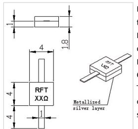
RF Solution offer a wide selection of Leaded Resistor for global customers. RFTXX-20RM0404 is a Leaded Resistor in Capacitance of 1.2 PF@100 $\Omega$ . It is made of high quality materials under a high standard, the Resistance Range of this product is XX  $\Omega$  (10-3000 $\Omega$ Customizable), Resistance Tolerance is ±5% and Temperature Coefficient Max is 150 ppm/°C. The component has a good working performance and stability, it is ideal for handling a Power of 20 W.
