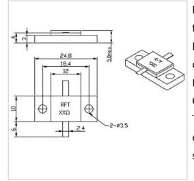
RF Solution offer a wide selection of Flanged Resistor for global customers. RFTXX-150RM2510 is a Flanged Resistor in Capacitance of 5.0 PF@100 $\Omega$ . It is made of high quality materials under a high standard, the Resistance of this product is XX  $\Omega$  (10~1000 $\Omega$ Customizable), Resistance Tolerance is ±5% and Temperature Coefficient Max is 150 ppm/°C. The component has a good working performance and stability, it is ideal for handling a Power of 150 W.
