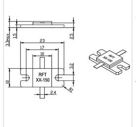
RF Solution offer a wide selection of Flanged Resistor for global customers. RFTXX-150RM2310 is a Flanged Resistor in Capacitance of 5.6 PF@100 $\Omega$ . It is made of high quality materials under a high standard, the Resistance of this product is XX  $\Omega$  (10~1000 $\Omega$ Customizable), Resistance Tolerance is ±5% and Temperature Coefficient Max is 150 ppm/°C. The component has a good working performance and stability, it is ideal for handling a Power of 150 W.
