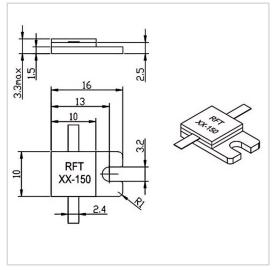
RF Solution offer a wide selection of Flanged Resistor for global customers. RFTXX-150RM1610 is a Flanged Resistor in Capacitance of 5.6 PF@100 $\Omega$ . It is made of high quality materials under a high standard, the Resistance of this product is XX  $\Omega$  (10~1500 $\Omega$  Customizable), Resistance Tolerance is  $\pm 5\%$  and Temperature Coefficient Max is 150 ppm/°C. The component has a good working performance and stability, it is ideal for handling a Power of 150 W.
