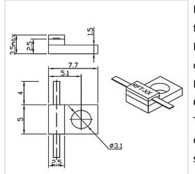
RF Solution offer a wide selection of Flanged Resistor for global customers. RFTXX-10RM7750 is a Flanged Resistor in Capacitance of 1.2 PF@100 $\Omega$ . It is made of high quality materials under a high standard, the Resistance of this product is XX  $\Omega$  (10~3000 $\Omega$ Customizable), Resistance Tolerance is ±5% and Temperature Coefficient Max is 150 ppm/°C. The component has a good working performance and stability, it is ideal for handling a Power of 10 W.
