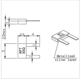
RF Solution offer a wide selection of Leaded Resistor for global customers. RFTXX-10RM5025C is a Leaded Resistor in Capacitance of 1.8 PF@100 $\Omega$ . It is made of high quality materials under a high standard, the Resistance Range of this product is XX  $\Omega$  (10-3000 $\Omega$ Customizable), Resistance Tolerance is ±5% and Temperature Coefficient Max is 150 ppm/°C. The component has a good working performance and stability, it is ideal for handling a Power of 10 W.
