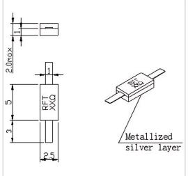
RF Solution offer a wide selection of Leaded Resistor for global customers. RFTXX-10RM2550 is a Leaded Resistor in Capacitance of 1.8 PF@100 $\Omega$ . It is made of high quality materials under a high standard, the Resistance Range of this product is XX  $\Omega$  (10-3000 $\Omega$  Customizable), Resistance Tolerance is  $\pm 5\%$  and Temperature Coefficient Max is 150 ppm/°C. The component has a good working performance and stability, it is ideal for handling a Power of 10 W.
