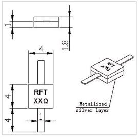
RF Solution offer a wide selection of Leaded Resistor for global customers. RFTXX-10RM0404 is a Leaded Resistor in Capacitance of 1.2 PF@100 $\Omega$ . It is made of high quality materials under a high standard, the Resistance Range of this product is XX  $\Omega$  (10-3000 $\Omega$  Customizable), Resistance Tolerance is  $\pm 5\%$  and Temperature Coefficient Max is 150 ppm/°C. The component has a good working performance and stability, it is ideal for handling a Power of 10 W.
