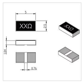
RF Solution offer a wide selection of Chip Resistor for global customers. RFTXX-10CR2550TA is a Chip Resistor in Resistance Range of XX  $\Omega$  (10~3000 $\Omega$  Customizable). It is made of high quality materials under a high standard, the Resistance Tolerance of this product is  $\pm 5\%$ , Substrate Material is BeO and Resistive Element is Thick Film. The component has a good working performance and stability, it is ideal for handling a Power of 10 W.
