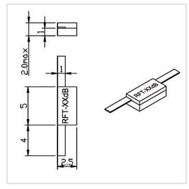
RF Solution offer a wide selection of Leaded Attenuator for global customers. RFTXX-10AM2505B-4 is a Leaded Attenuator in Frequency Range of DC~4.0 GHz. It is made of high quality materials under a high standard, the Attenuation Value of this product is **10.5** dB@01,02,03,04,07,10 dB@11 dB, Attenuation Tolerance is  $0-0.2\sim+0.8$  dB $2\pm0.6$  dB $3\pm0.8$  dB and VSWR Max is 1.20. The component has a good working performance and stability, it is ideal for handling a Rated Power of 5 W.
