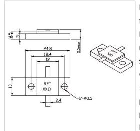
RF Solution offer a wide selection of Flanged Resistor for global customers. RFTXX-100RM2510B is a Flanged Resistor in Capacitance of 4.0 PF@100 $\Omega$ . It is made of high quality materials under a high standard, the Resistance of this product is XX  $\Omega$ (10~1000 $\Omega$  Customizable), Resistance Tolerance is ±5% and Temperature Coefficient Max is 150 ppm/°C. The component has a good working performance and stability, it is ideal for handling a Power of 100 W.
