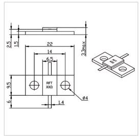
RF Solution offer a wide selection of Flanged Resistor for global customers. RFTXX-100RM2295 is a Flanged Resistor in Capacitance of 3.9 PF@100 $\Omega$ . It is made of high quality materials under a high standard, the Resistance of this product is XX  $\Omega$  (10~1500 $\Omega$  Customizable), Resistance Tolerance is  $\pm 5\%$  and Temperature Coefficient Max is 150 ppm/°C. The component has a good working performance and stability, it is ideal for handling a Power of 100 W.
