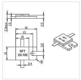
RF Solution offer a wide selection of Flanged Resistor for global customers. RFTXX-100RM1610 is a Flanged Resistor in Capacitance of 5.6 PF@100 $\Omega$ . It is made of high quality materials under a high standard, the Resistance of this product is XX  $\Omega$  (10~1500 $\Omega$  Customizable), Resistance Tolerance is  $\pm 5\%$  and Temperature Coefficient Max is 150 ppm/°C. The component has a good working performance and stability, it is ideal for handling a Power of 100 W.
